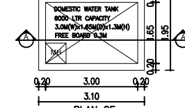
PLAN OF DOMESTIC WATER SUMP
