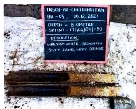
Plate – 3 Soil Sample Collected by conducting SPT in BH-03 Location
