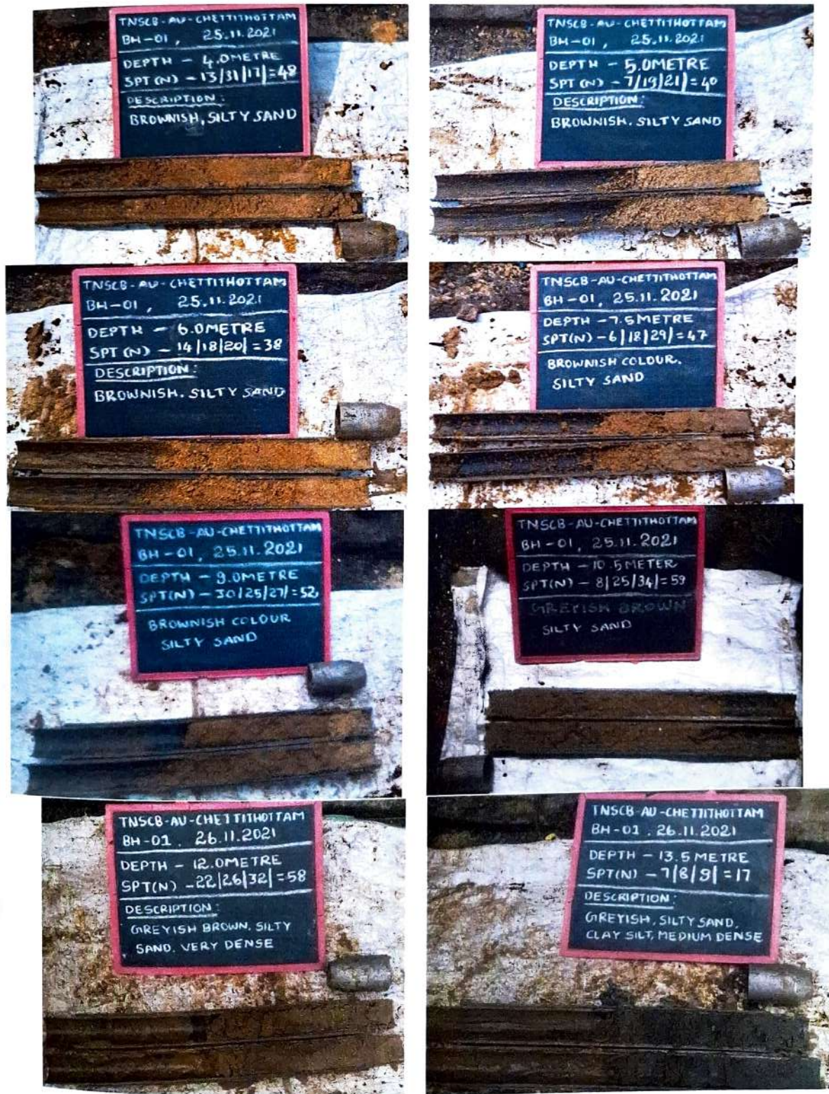
Plate – 1 Soil Sample Collected by conducting SPT in BH-01 Location
