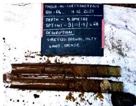
Plate – 4 Soil Sample Collected by conducting SPT in BH-04 Location
