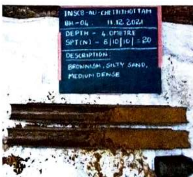
Plate – 4 Soil Sample Collected by conducting SPT in BH-04 Location
