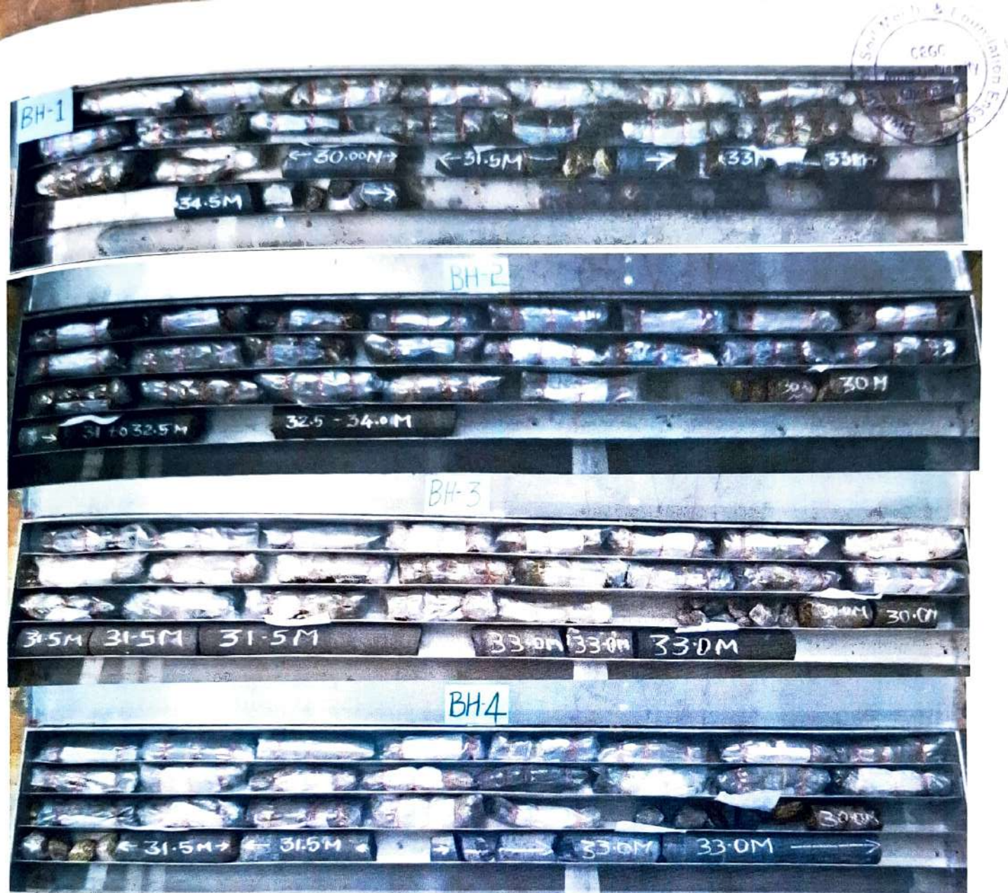
Plate 2 View of Soil / Rock Samples collected in 4 borehole locations of the proposed site
