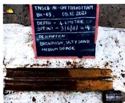
Plate – 3 Soil Sample Collected by conducting SPT in BH-03 Location
