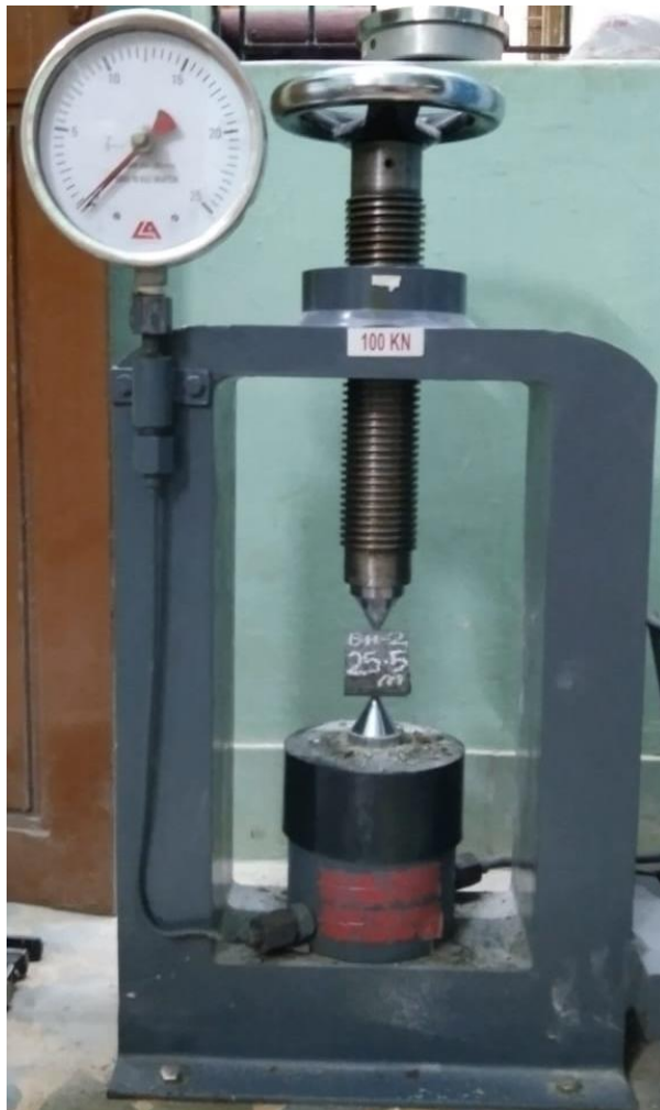
Plate 3 View of Rock Samples tested for Point Load Strength Index and Unconfined Compression Strength
