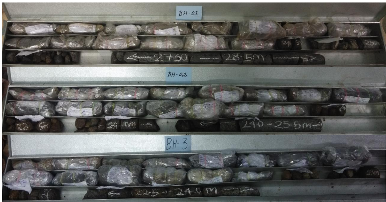
Plate 2 View of Soil / Rock Samples collected in 3 borehole locations of the proposed site
