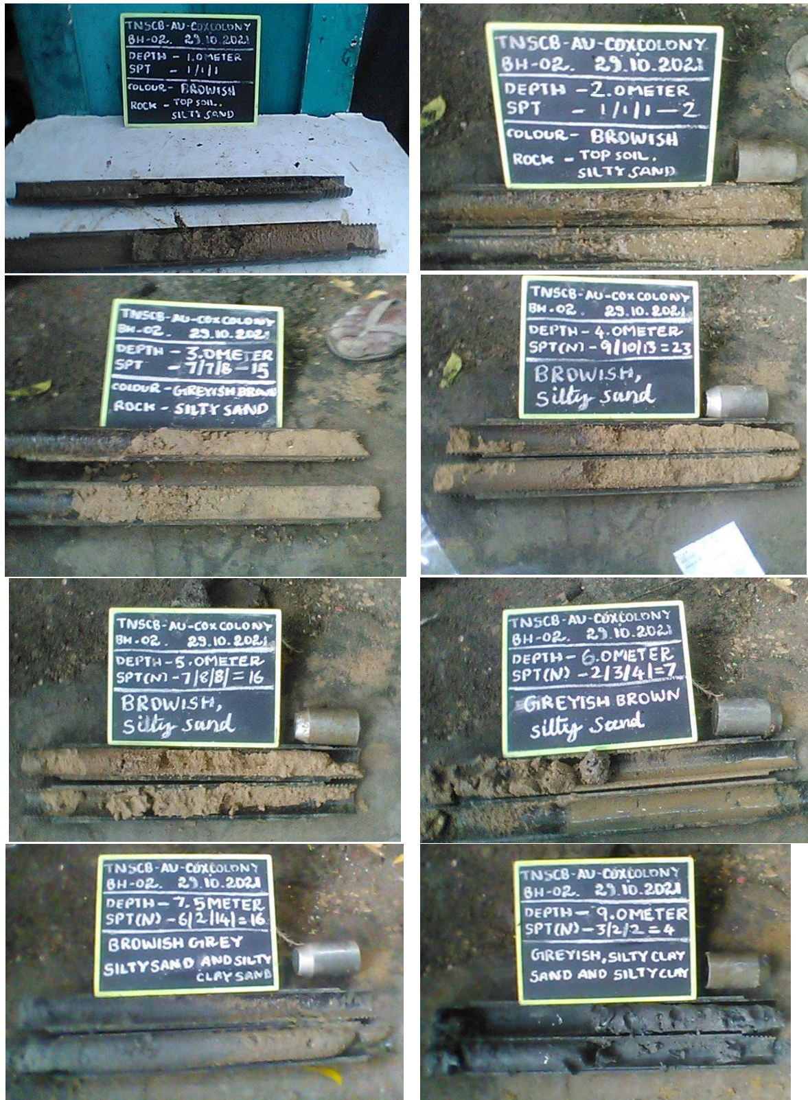
Plate – 2 Soil Sample Collected by conducting SPT in BH-02 Location
