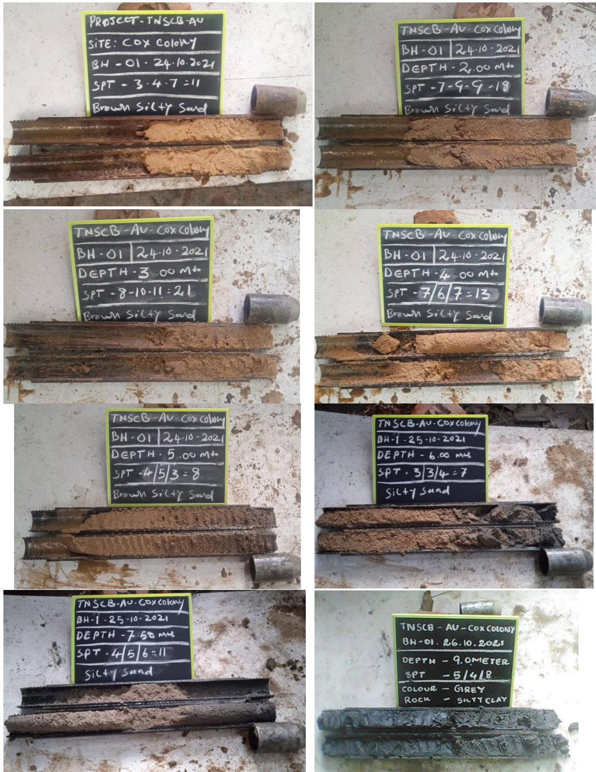
Plate – 1 Soil Sample Collected by conducting SPT in BH-01 Location
