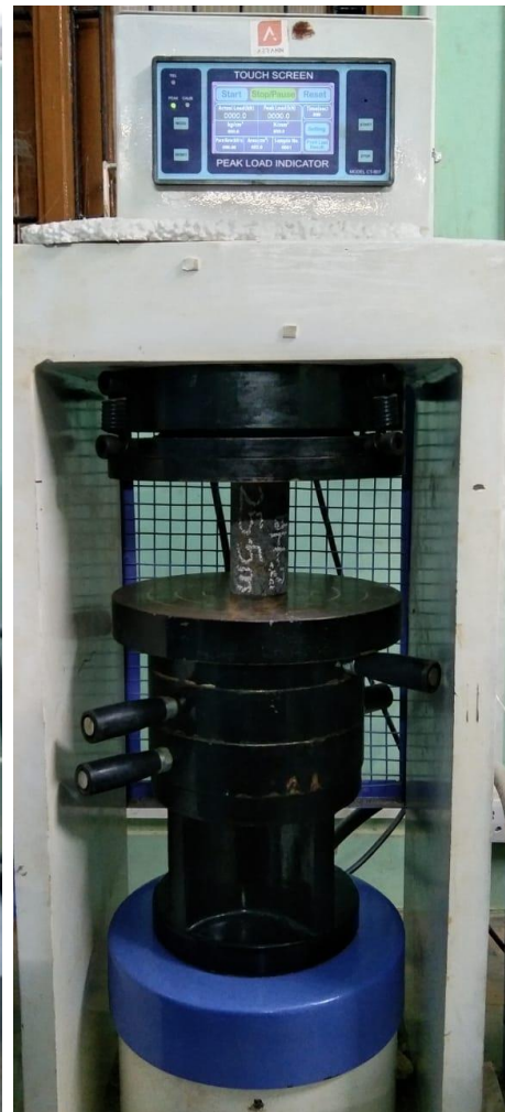
Plate 3 View of Rock Samples tested for Point Load Strength Index and Unconfined Compression Strength
