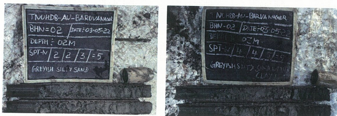
Plate – 2 Soil / Rock Samples Collected in BH-02 Location
