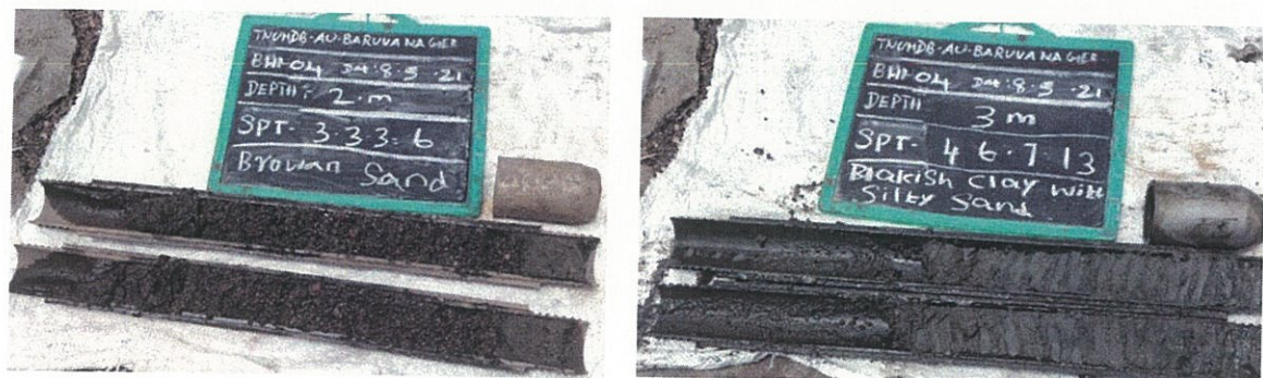
Plate – 4 Soil / Rock Samples Collected in BH-04 Location
