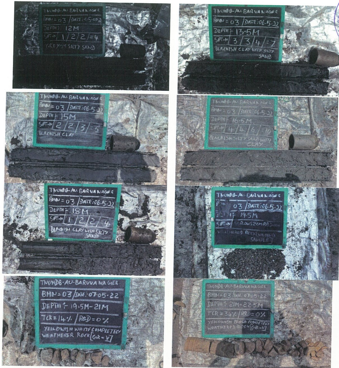
Plate – 4 Soil / Rock Samples Collected in BH-04 Location
