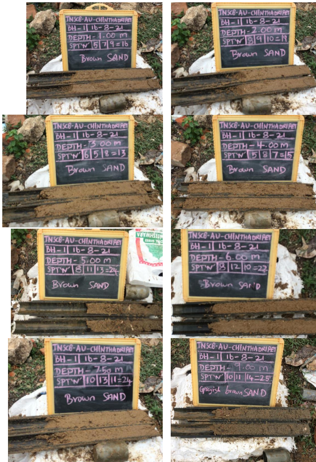
Plate – 1 Soil Sample Collected by conducting SPT in BH-01 Location
