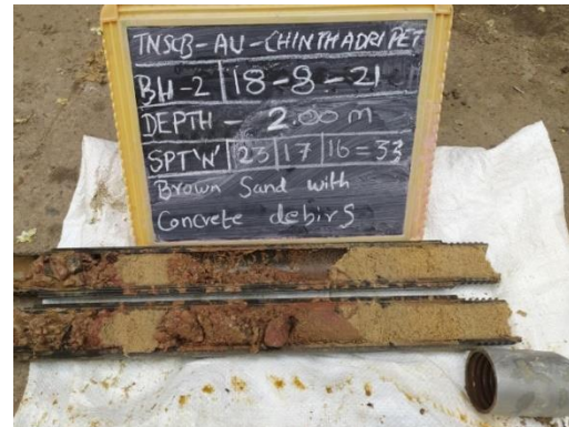
Plate – 2 Soil Sample Collected by conducting SPT in BH-02 Location
