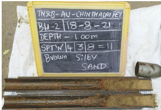
Plate – 2 Soil Sample Collected by conducting SPT in BH-02 Location
