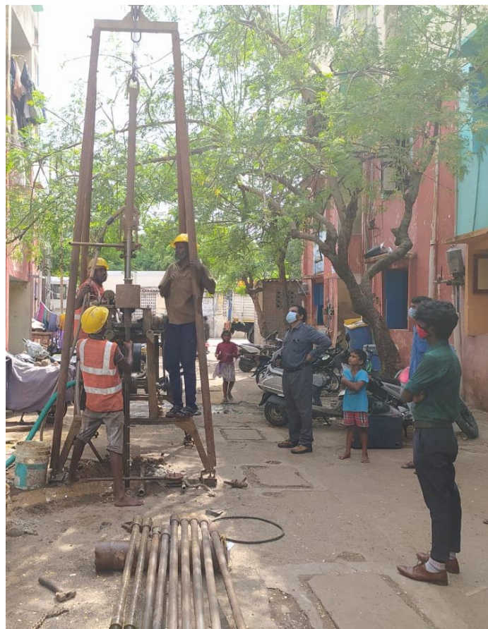
Plate 1 SPT test is in progress at the Reconstruction of Dilapidated Slum Tenements (S+6 Floors) at Chindadripet Scheme in Corporation Division 62, Zone V of Greater Chennai Corporation.
