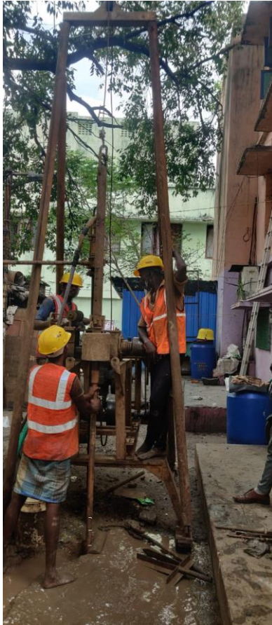
Plate 1 SPT test is in progress at the Reconstruction of Dilapidated Slum Tenements (S+6 Floors) at Chindadripet Scheme in Corporation Division 62, Zone V of Greater Chennai Corporation.
