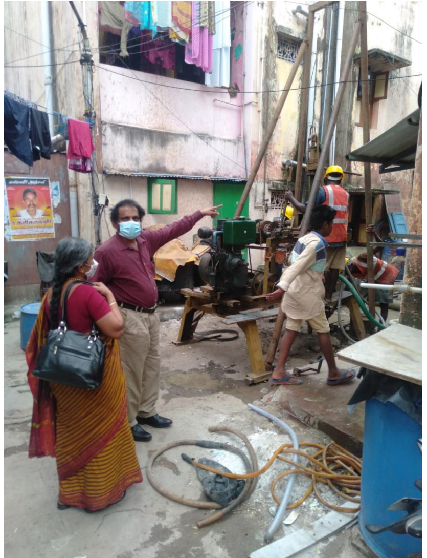
Plate 1 SPT test is in progress at the Proposed Reconstruction of Dilapidated Slum Tenements (S + 5 Floors) at Ellispuram Tenemental Scheme in Corporation Division 59, Zone V of Greater Chennai Corporation.
