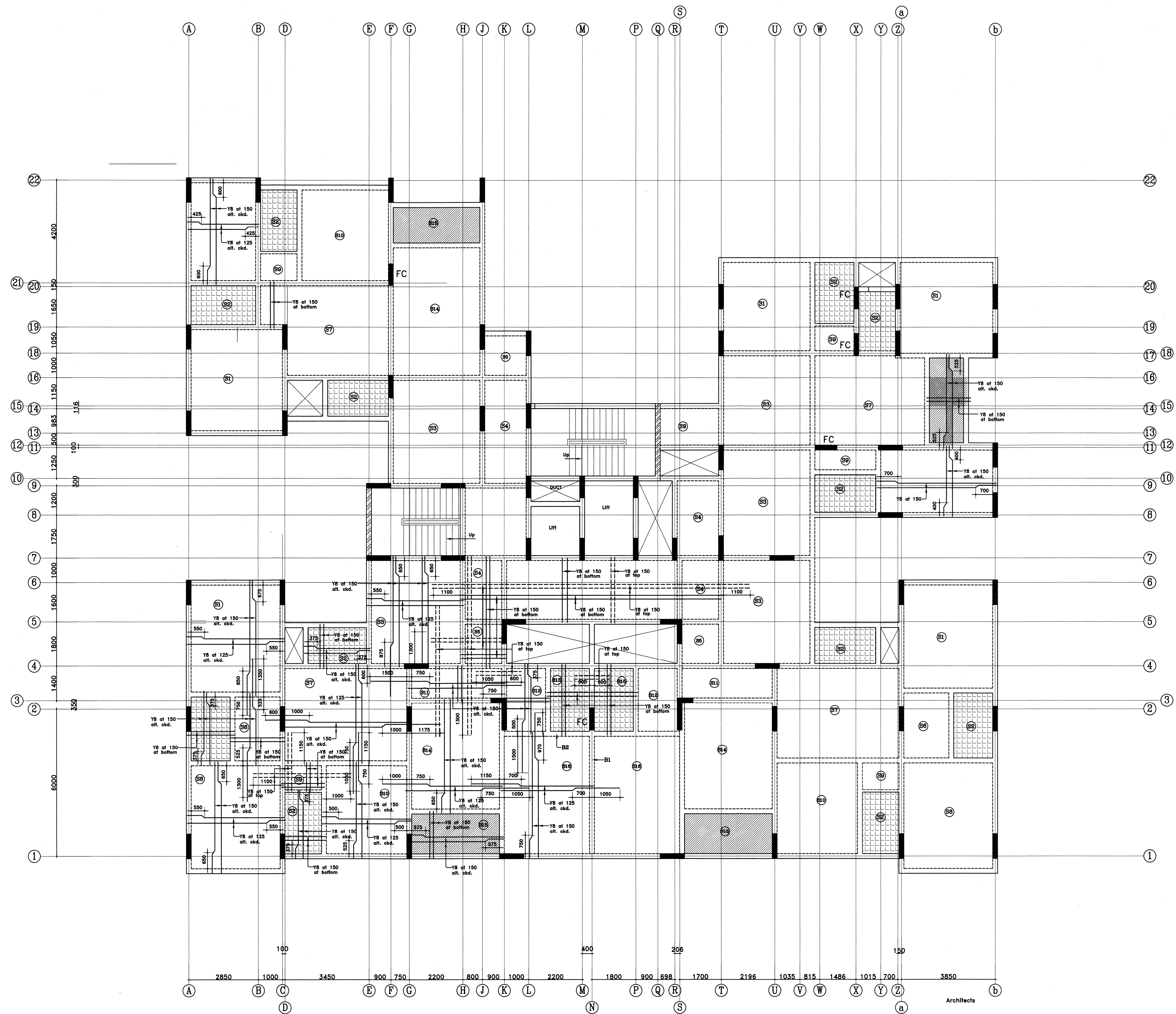
Lay - out of Typical floor slabs & beams
