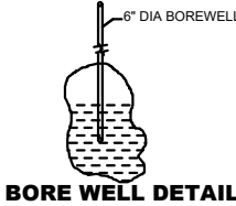
BORE WELL DETAIL
