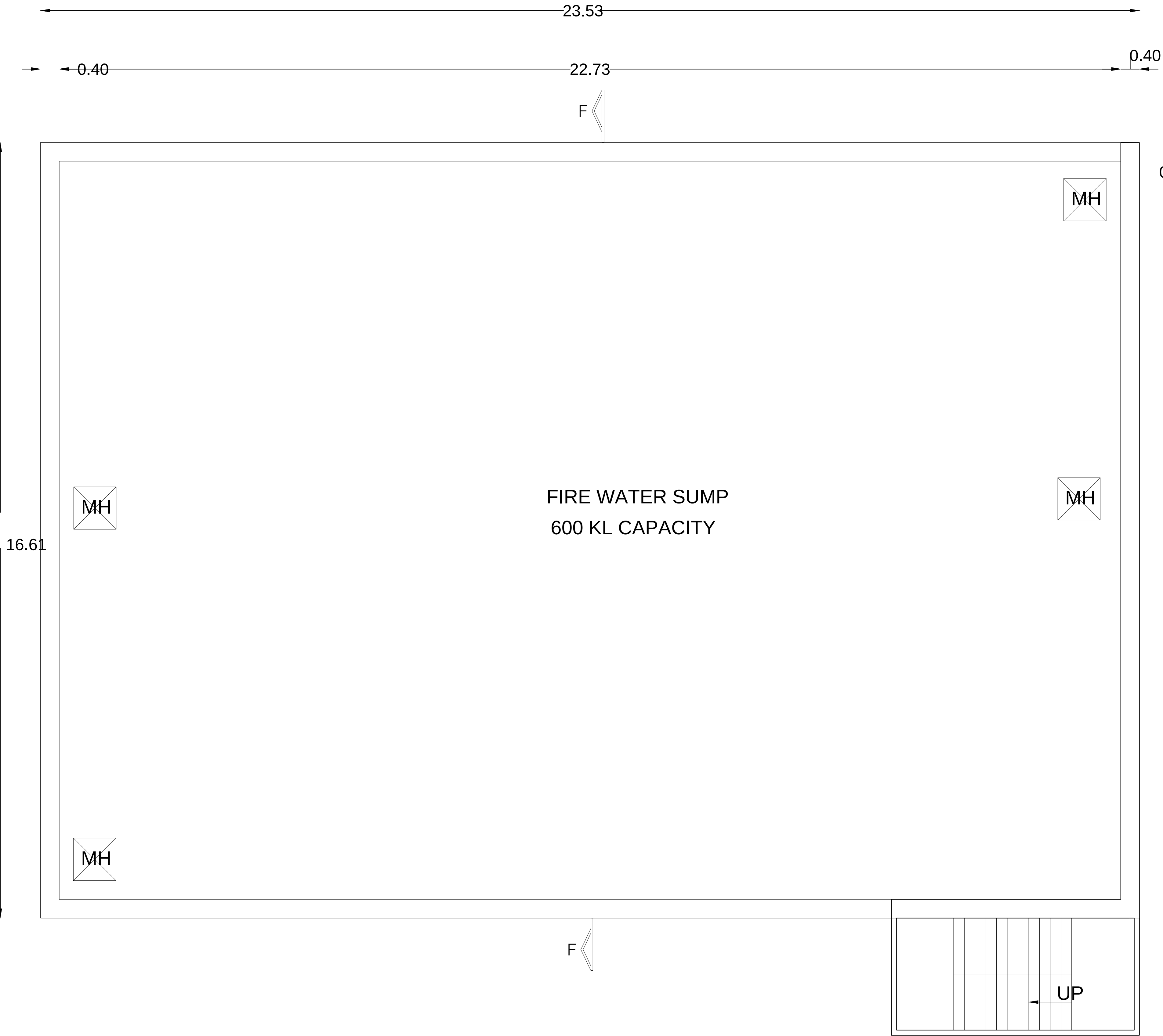
GROUND FLOOR PLAN MAIN RAW WATER SUMP
