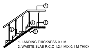
SECTION OF STAIRCASE
