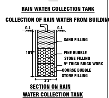
RAIN WATER COLLECTION TANK COLLECTION OF RAIN WATER FROM BUILDING
