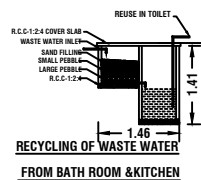
RECYCLING OF WASTE WATER
