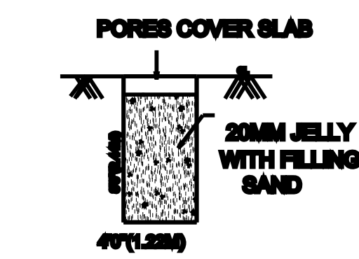
RAIN WATER HARVESTING UNIT
