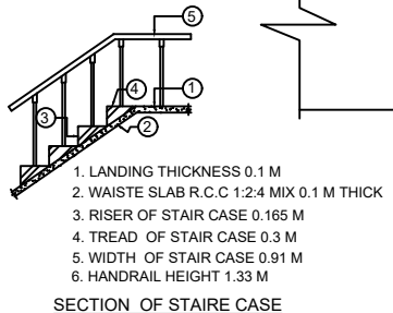
SECTION OF STAIRCASE
