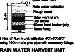
RAIN WATER HARVEST UNIT
